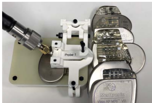
Figure 2: This test fixture was constructed to allow direct measurement of the impedance between an IPG's header connector block and Can. Also shown are the IPGs modified to provide direct access to terminal blocks to allow this measurement.
